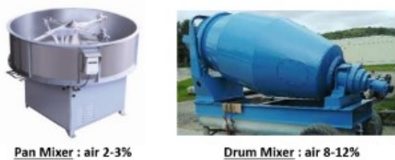
Figure 19 Air content of concrete mixed with pan and drum mixer
