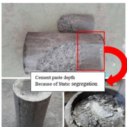
Figure 12 Split concrete cylinder section that has static segregation.
