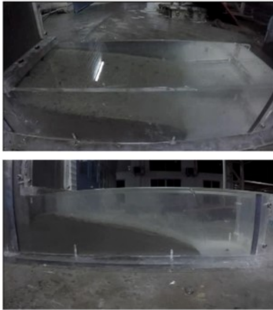
Figure 14 L-Box testing with water
